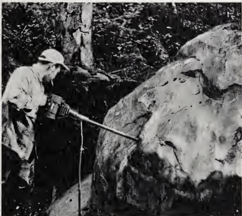
Diamond-drill sampling of multi-ton jade boulder on the side of Ogden Mountain, B.C.
